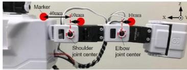
Fig.1 Reflective marker positions and laboratory coordinate system.
