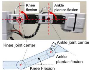
Fig. 2 Correspondence between robot and human lower limb joints.
